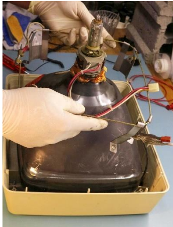
Figure 84 VT220, retirer les composantes © HE-Arc, N. Nydegger, 2019
