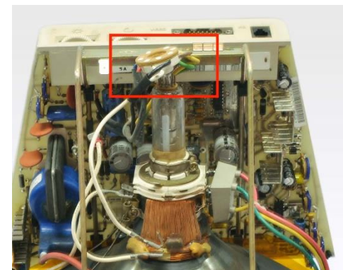
Figure 92 VR201, retirer la boucle de la cathode © HE-Arc, N. Nydegger, 2019
