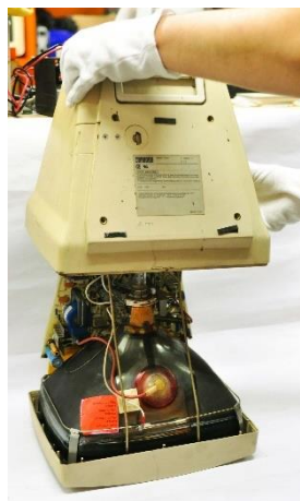
Figure 87 VR201, soulever le boîtier © HE-Arc, N. Nydegger, 2019
