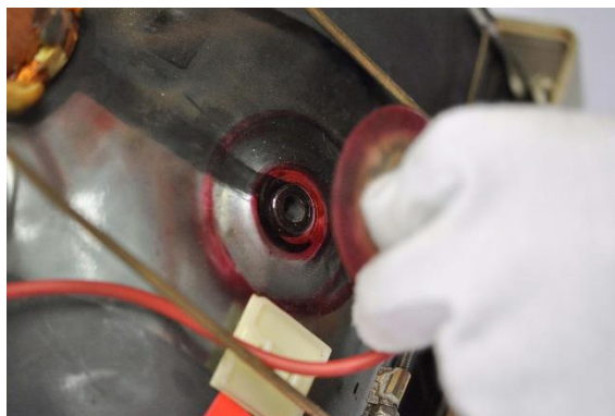
Figure 93 VR201, retirer le bouton d'anode © HE-Arc, N. Nydegger, 2019
